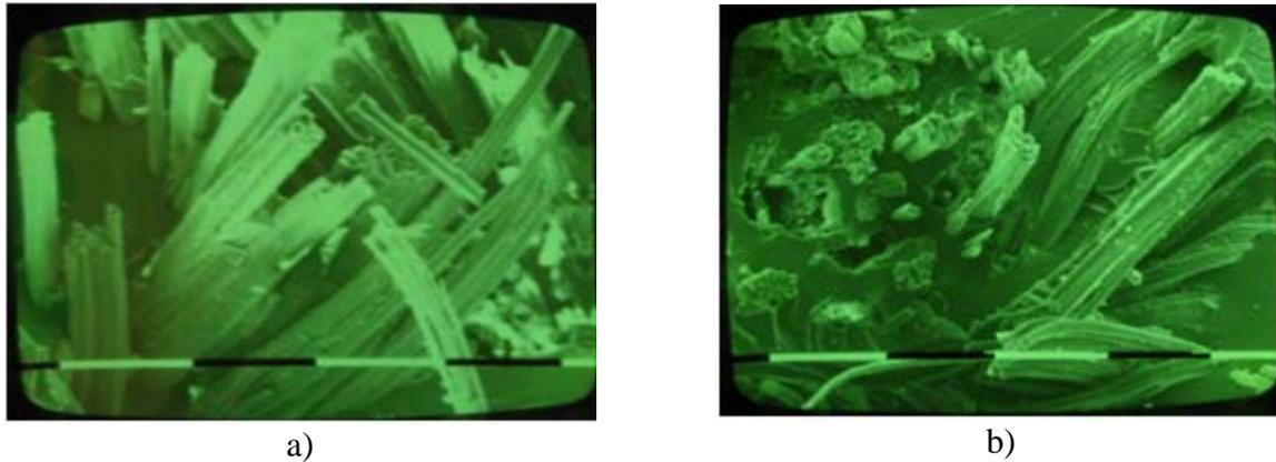
Fig. 2 SEM pictures of tensile fractured surface of composites, a) natural: b) bleached.
