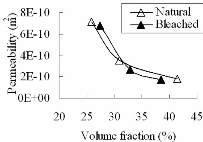
Fig. 1 Effect of fiber volume fraction (%) on permeability of jute fabrics (using corn syrup).
